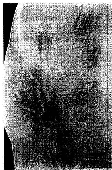
Fig. 3. The electron micrograph of the bacterial cellulose after the hydrothermal treatment under NaOH.
